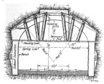
FIG. 10. TIMBERING IN MAIN TUNNEL
