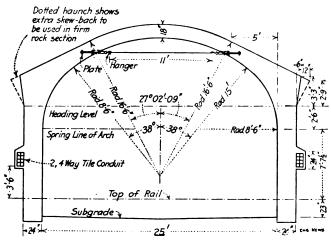
FIG. 4. TYPICAL SECTION OF MAIN TUNNEL
