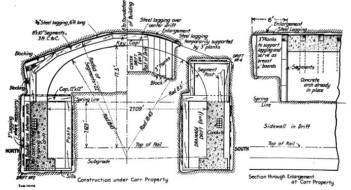
FIG. 9. TUNNEL TIMBERING UNDER CARR PROPERTY
