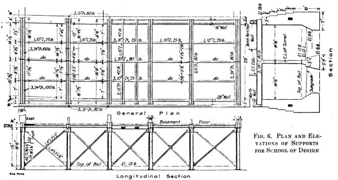
as far as the face of the School of Design and thence to the portal under the portion of that building carrying the least load. One tunnel sidewall from subgrade to spring line was then concreted in the drift under the Carr property.
